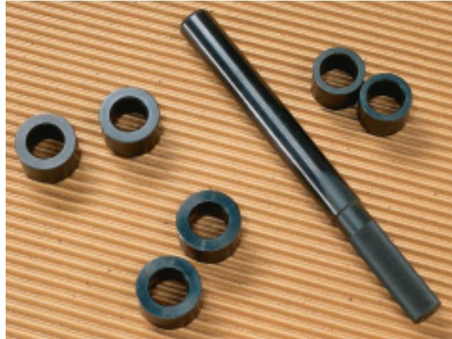
Photo 24, Spicer Alignment Bar, Quick Disconnect Style
